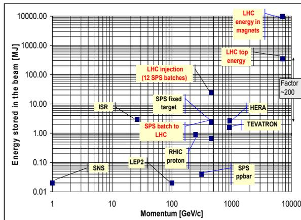
Figure 1. Energy stored in LHC beams and magnets compared with other accelerators
