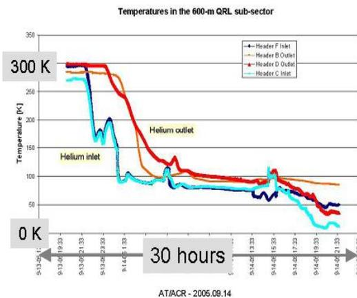
Figure 5: Cooling down of a 600 m long section of the cryogenic distribution line
