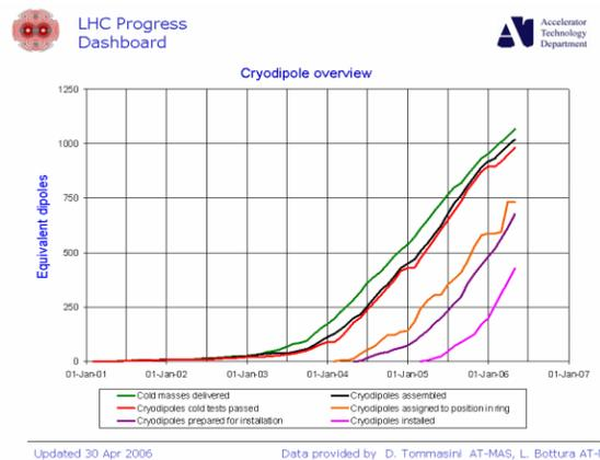
Figure 3: LHC dashboard - progress of construction and installation of cryodipole magnets
