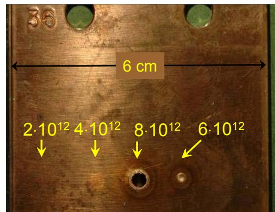
Figure 6: Controlled damage of a stack of metal plates with the SPS 450 GeV beam
