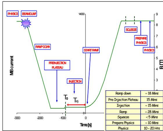
Figure 7: LHC operational cycle
