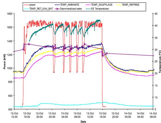
Figure 4: Power consumption during short circuit tests
