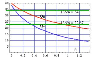
Figure 2. Betatron tune variation versus momentum deviation  $\delta$  for the AGS-FFAG with range of stability according to S.Y. Lee between green lines.
