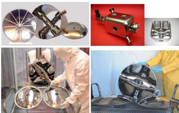
Figure 4: Multi-spoke cavities developed for RIA (top-left and bottom) and for HIPPI (top-right).
