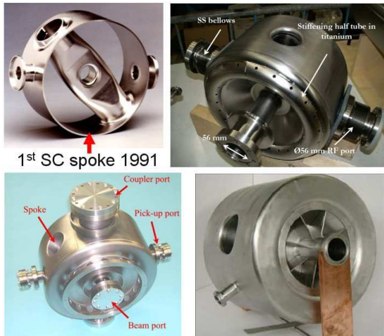
Figure 3: Single-spoke cavities developed for SDI (top-left), EURISOL (top-right), AAA (bottom-left) and XADS (bottom-right).
