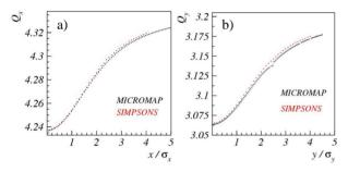
Figure 2: Comparison of a) transverse horizontal and b) vertical tunes.
