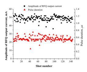
Figure 6: Shot-to-shot fluctuations of output RFQ current amplitude and pulse duration (extraction potential -60 kV, RF voltage amplitude -120 kV).
