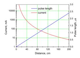
Figure 1: Dependences of  ${}^{12}C^{4+}$  ion current into 1 cm<sup>2</sup> and corresponding ion pulse duration on the distance from the target.
