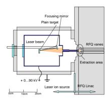
Figure 2: Lay-out of DPIS experiment.
