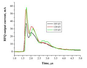
Figure 4: Time dependences of RFQ output currents for different RF voltage amplitudes.
