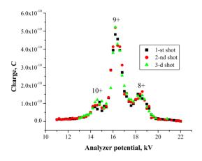
Figure 5: Charge state distribution (extraction potential – 60 kV, RF voltage amplitude – 120 kV, 3 shots for each analyzer potential).
