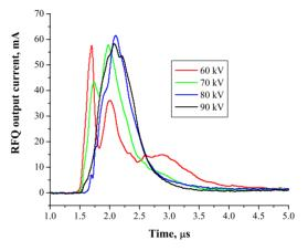
Figure 3: Time dependences of RFQ output currents for different extraction potentials.
