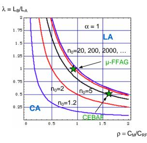
Figure 3. Plot of length ratio  $\lambda = L_B/L_A$  versus cost ratio  $\rho = C_M/C_{RF}$  for different threshold value of number of revolutions  $n_0$  for which the two scenarios A and B have about the same cost.
