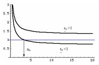
Figure 2. Cost ratio r vs. number of revolutions in the CA
