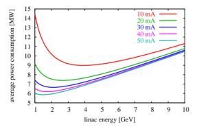
Figure 1: Av. SPL RF power at 50 Hz, 4 MW beam power for various pulse currents, top to bottom:  $10 \rightarrow 50$  mA.
