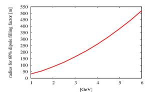
Figure 3: Minimum arc radius for a 4 MW beam, assuming 0.1 W/m stripping losses and a 60% dipole filling factor.
