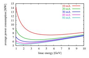
Figure 2: Av. SPL RF power at 25 Hz, 4 MW beam power for different pulse currents, top to bottom:  $10 \rightarrow 50$  mA.
