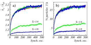
Figure 7: a) Emittance growth for  $\Sigma = 1/4$  (green),  $\Sigma = 1/8$  (blue), with  $Q_{z0} = 10^{-3}$  and for  $Q_{z0} \rightarrow Q_{z0}/\Sigma$  (all overlapping). b) % of halo particles. The meaning of the curves is as in a).
