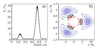
Figure 8: a) Asymmetry of the invariant in one synchrotron oscillation; b) Transverse islands for  $\delta Q_c = +0.01$  (red),  $\delta Q_c = -0.01$  (blue), corresponding to the loss/increase of particle momentum.
