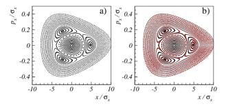
Figure 6: a) Phase space for  $\Sigma = 1$  (for standard parameters). In b) phase space for  $\Sigma = 1/4$  (red orbits) overlapped with orbits in a) for better comparison.
