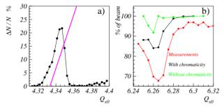
Figure 9: a) beam loss induced by chromaticity; b) New beam loss prediction for the PS-experiment: the black curve gives the simulated beam loss in presence of chromaticity.
