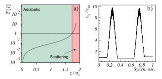
Figure 2: a) Adiabaticity parameter T and b) evolution of the single particle invariant in an adiabatic regime for the same test particle of Fig. 1.
