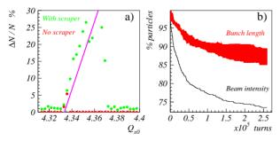
Figure 4: a) Beam loss induced by trapping/scattering of particles (green markers), in red markers beam loss by shrinking of the DA (no scraper); b) Bunch intensity/length evolution vs. storage time for  $Q_{x0} = 4.3525$ .
