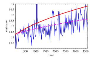
Figure 5: Horizontal 95% normalized emittance  $[\mu m]$  vs time [sec]. Exact Martini's model: pink (dash) line; 50% higher "enhanced" transverse growth rate: red (solid) line. Measurements: blue solid line.
