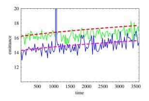
Figure 4: Horizontal 95% normalized emittance  $[\mu m]$  vs time [sec] for two bunch intensities:  $2.9 \times 10^9$  (upper curve) and  $1.4 \times 10^9$  Cu ions. Dash lines - simulations; solid lines - measurements.
