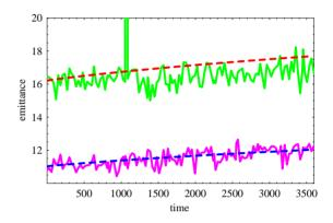
Figure 2: Horizontal and vertical 95% normalized emittance  $[\mu m]$  vs time [sec] for bunch intensity  $2.9 \times 10^9$  Cu ions. Measured emittance: top green curve (horizontal), bottom pink curve (vertical). BETACOOL simulation using Martini's model: top red dash line (horizontal), blue dash line (vertical).
