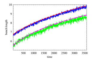
Figure 3: Growth of FWHM bunch length [ns] vs time [sec] for two bunch intensities:  $2.9 \times 10^9$  (upper curve) and  $1.4 \times 10^9$  (lower curve) Cu ions. Dash lines - simulations.
