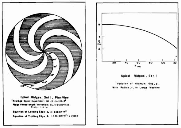
Fig. 17. Plan view of "low-field" poleface
