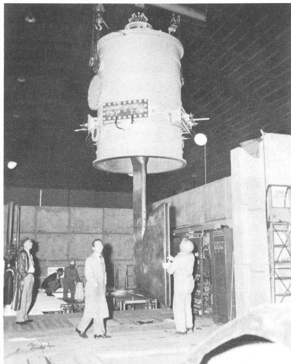
Fig. 156. The notched shape of the dee of the 90-in. cyclotron reduces the voltage taper along the dee edge to about 2%.
