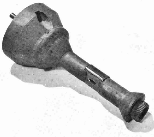
Fig. 15 Ion source with tantalum insert.
