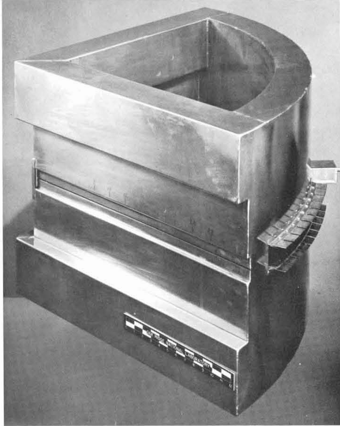
Fig. 5 Model of Me^2 coaxial cavity.
