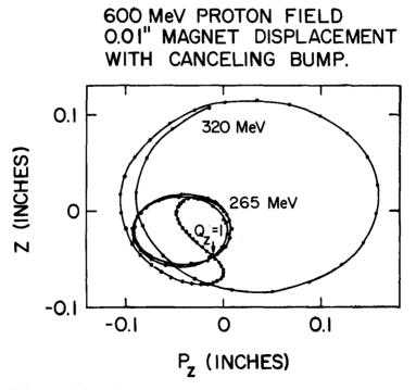
Fig. 5. Repeat of the acceleration run of Fig. 4 but with the median plane correcting coil turned on and roughly optimised. (Note the change in scale relative to Fig. 4)
