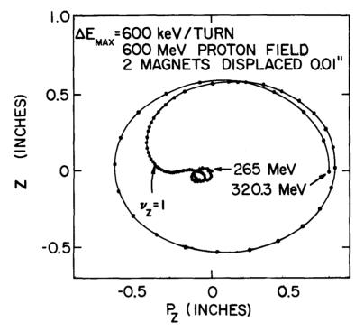
Fig. 4. Plot of Z vs  $P_Z$  on successive revolutions for an orbit accelerated through the  $Q_Z = 1$  resonance. Two magnets 180° apart are displaced up and down by 0.01 in respectively
