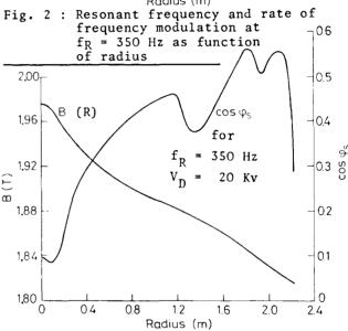
Fig. 3: Magnetic field of SC2 and the cosine of the synchronous phase angle for  $f_R$  = 350 Hz and  $V_D$  = 20 kV as function of radius
