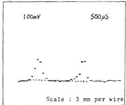
Fig. 8: Horizontal and vertical profiles of the extracted proton beam, measured with a vacuum wire chamber
