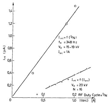
Fig. 5: Internal beam as function of RF duty cycle and ion-source arc current
