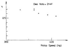
Fig. 7: Extraction efficiency as function of dee-voltage and pulse repetition rate
