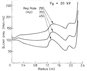
Fig. 4: Bucket area as function of radius for  $V_D$  = 20 kV and different pulse repetition rates
