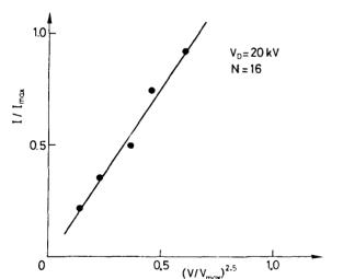
Fig. 6: Internal beam as function of dee voltage
