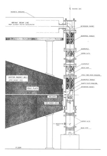
1m AXIAL INJECTION SYSTEM 1m FOR THE RING CYCLOTRON 08-72
