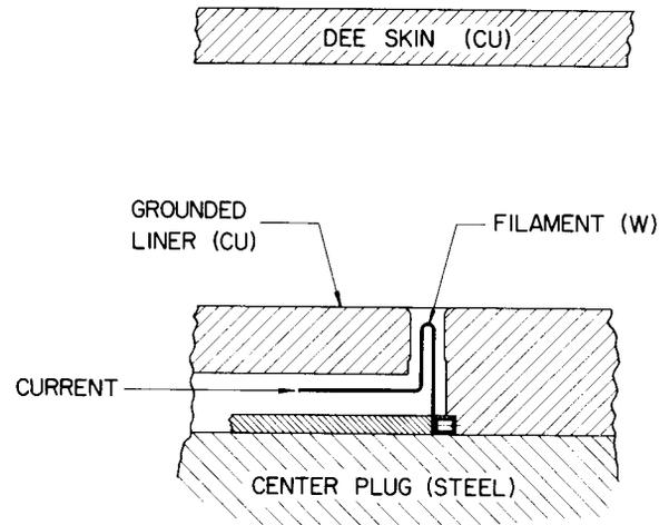
Fig. 1.--Layout of one electron source in the cyclotron. The support for the non-grounded side of the filament is not shown.
