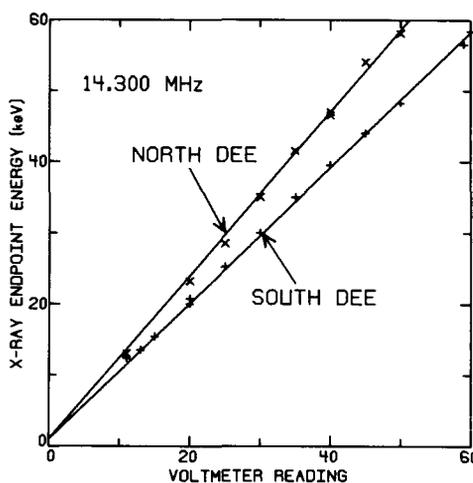
Fig. 3.--Calibration data for north and south dee voltmeters at 14.300 MHz. The straight lines are fitted by least squares. Standard deviations are 0.78 keV for the north dee and 0.50 keV for the south dee. Note that the voltmeter reading is treated as dimensionless, so both the slope and the intercept of each line can be expressed in keV.
