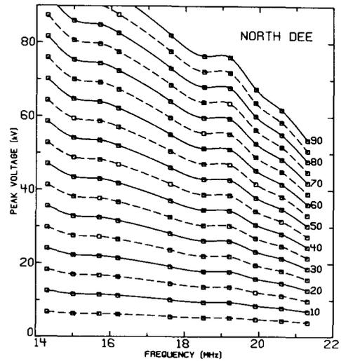
Fig. 6.--North dee voltage as a function of frequency with the voltmeter reading as the parameter (5 unit contours).
