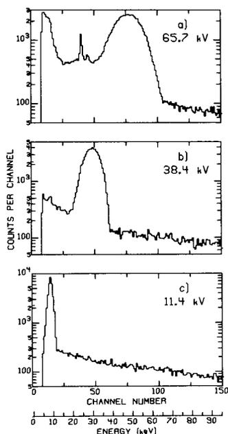
Fig. 2.--Typical X-ray spectra for three different peak voltages. The endpoint can be estimated to within about 1 channel (.639 keV). Absorber thickness: a) 1.1 mm; b) 0.25 mm; c) none. (See text).
