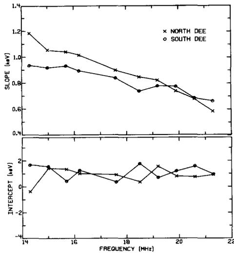
Fig. 4.--Frequency dependence of the voltmeter calibration parameters (slope and intercept of the linear fit). Both parameters were allowed to vary.
