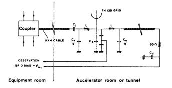
Fig.9: HF power amplifier matching filter.
