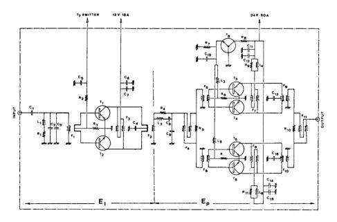
Fig.1 : 100 W. solid-state wide-band amplifier module .
