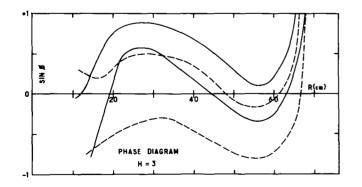
Figure 8 - Phase diagrams. Solids curves : wrong trimming, with 1 mm slit. Dashed lines : correct trimming, no slit.
