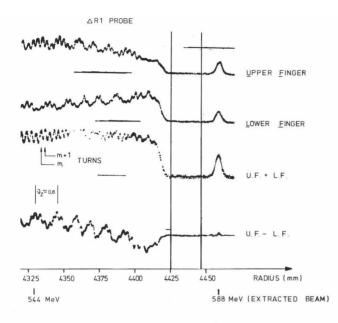
Plots obtained with the  $\Delta R1$  probe. The two vertical lines simulate the thickness of the septum coil of the extraction magnet (AHA). This probe can be used with a 100  $\mu A$ beam without disturbing the beam users.
