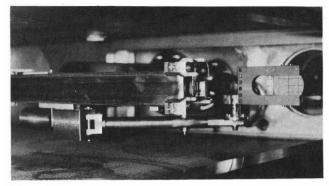
View of the focusing magnet (FM) built into the SIN ring cyclotron. Four thermal sensors (thermocouples attached to molybdenum fingers) are mounted at the entrance of the 20 mm diameter channel. A quartz with a 1 cm x 1.4 cm ruled grid can be flipped from the position shown here into the path of the extracted beam from the control room.
