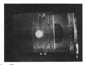
Fig. 27 Picture taken from a TV monitor showing a 590 MeV, 1  $\mu A$  beam at the entrance of the FM. The beam diameter is approx. 1 cm.
