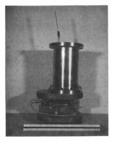
Radial scanner (RS) used at the SIN ring cyclotron. The indirectly water-cooled molybdenum finger sweeps across the accelerated beam giving the pattern shown in the following figure. The radial thickness of the finger is 0.5 mm. The diagnostic signal is derived from fully stopped protons plus secondary emission electrons. This scanner is an adaption of the profile monitors used in the SIN beam transport lines<sup>12</sup>.
