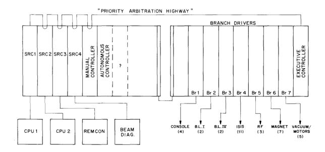
Fig. 2. System crate configuration. (The numbers in brackets indicate the number of crates currently on each branch.)
