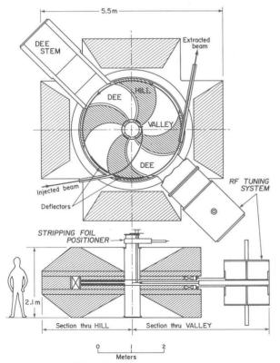
Fig. 3. The 400 N booster cyclotron.
