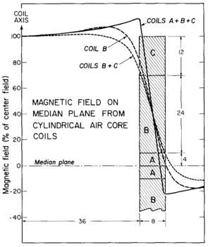
Fig. 6. Magnetic field of several coil combinations.
