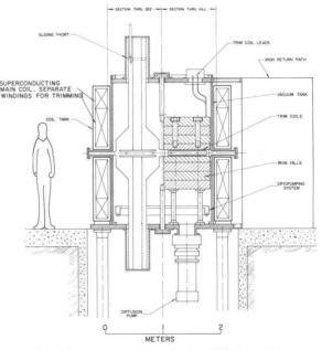
Fig. 5. Elevation view of the 400 S cyclotron.
