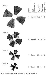
Fig. 2. Four cyclotron structures with the same K value or bending strength.
