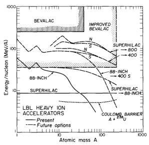
Fig. 1. Performance predictions for present and possible future LBL heavy ion accelerators.
