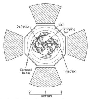
Fig. 4. Plan view of the 400 S cyclotron.
