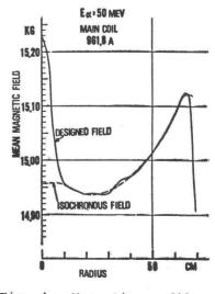
Fig. 4. Magnetic profile of radial direction.
