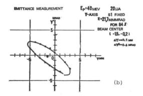
Figs. 6a. Vertical emittance of & 6b. protons at 20 µA, 40 MeV.
