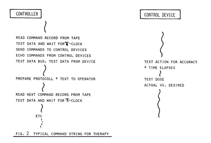
If any of the parameters has to be changed the appropriate command will be transferred from the controller to the control device for execution. The internal structure and speed of the data bus (ROAD) allows practically in the same time the recollection of the commands for echo-checking. Any type of transmission error might be detected and indicated within milliseconds.
