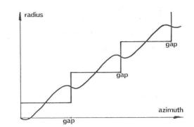
$\underline{Figure~2}$  : Accelerated orbit with minimum oscillation in a two gap or two dee geometry.
