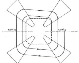
Figure 3 : Lozenge shape of the accelerated orbit in a two dee four sector SSC.
