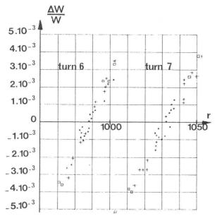
Figure 1 : Simulated  $r-\Delta W$  distribution of the particles after 6 and 7 turns. At such a place, it is possible to cut down the bunch length from  $\pm$  7.5° to  $\pm$  3° with a slit or a target between two turns
