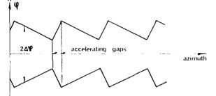
Figure 4 : Bunch length variation around a double gap two dee SSC. The amplitude of variation is proportional to the parameter A (here A = 0.4). The bunches are assumed matched in r,r', **P**-space at mid-valley asimuth.
