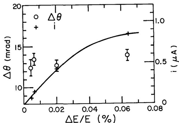
Fig. 5. Beam divergence angle ( $\Delta\theta$ ) and intensity ( $i$ ) vs. energy spread, controlled by the width of the analyzing slit. The energy spread of the entire beam was about .07%. There is no detectable change in beam divergence as the energy spread is reduced by a factor of 10.
