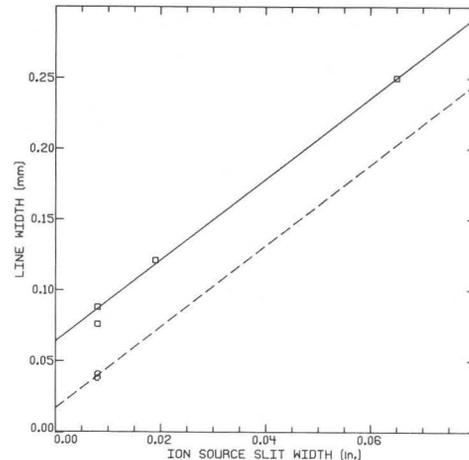
Fig. 4. Line width of image in spectrograph focal plane vs. ion source slit width. Dashed line is drawn with same slope as solid line. In the absence of aberrations and instrumental broadening effects, the line would pass through the origin if an image is formed.
