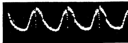
Fig. 3: Time structure of the extracted beam using the Kim Coil.
