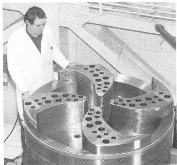
Fig. 6 The upper flutter pole assembly showing the 2 mm thick shims and the trim rod holes.
