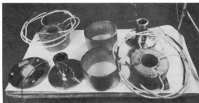
Fig. 4. One of two upper Glaser lenses of vertical line, disassembled.
