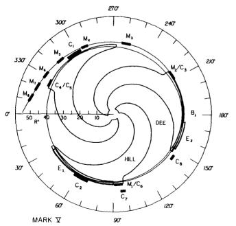
Fig. 1. Section view of the median plane of the K1200 cyclotron. For scale, the outside diameter of the cryostat, the largest circle shown, is 2.9 m. The outside diameter of the steel yoke (not shown) is 4.4 m.
