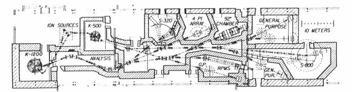
Fig. 2. The highbay floorplan of the complete NSCL Phase II Facility as presently planned; showing the two cyclotrons, the ion source switchyard, the beam transport system to deliver the beam from either cyclotron to any experimental area, and the various experimental devices.
