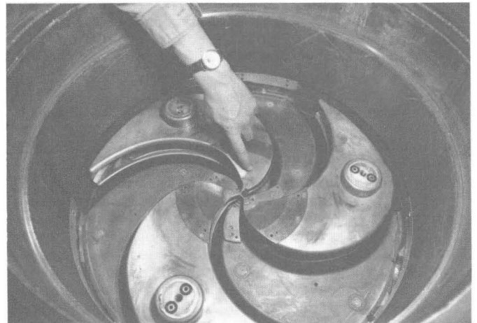
FIG. 6 -- Photograph of the K100 medical cyclotron with the upper pole cap raised to display the dees and lower pole tips.
