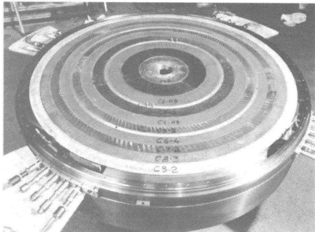
Fig.6. Trim coils in the stage of completion
