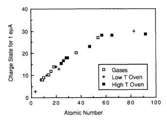
4. Charge states for 1 eµA intensity from the ECR source for gas and solid material feed.
