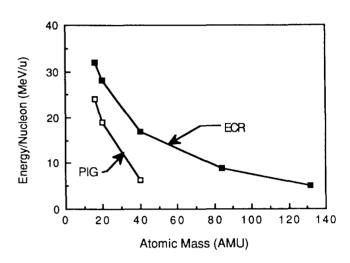
1. Energy vs. mass using PIG and ECR sources, with 10<sup>10</sup> particles/sec cyclotron external beam.
