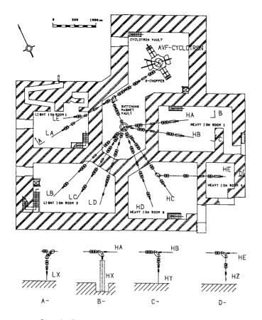
Fig. 2. The layout of the beam transport system for the cyclotron
