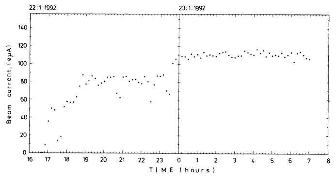
Fig. 3 The record of a target current during irradiation.
