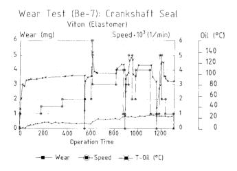
Fig. 5: .The wear behavior of the Be-7 labelled Viton (Elastomer) seal of the crankshaft in an engine (Audi V 6, 24 Valves) at different speed and oil temperature, was measured in a 24 h wear test and is demonstrating the effectiveness of RTM application.
