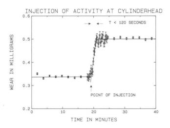
Fig. 7: In case of the activity injection into the cylinder head of the running engine, simulating wear occuring at the camshaft, the reactivity decreased to 120 sec..
