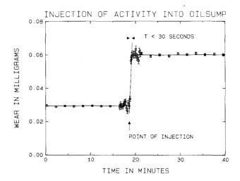
Fig. 6 :.For the demonstration of the sensivity and reactivity of RTM wear diagnosis a definite activity - representing 30  $\mu$ g wear mass - was injected in the oil sump of the operated engine on the KfK test bench. The applied concentration measurement device registered the full wear mass 30 sec after the injection. A wear mass down to 10  $\mu$ g - corresponding to a linear wear of several nanometers - can distinctly be resolved.
