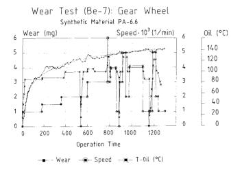
Fig. 4 : The wear behavior of the Polyamid gear over operation time at variated speed and oil temperature in an Audi engine is demonstrating the advantage of RTM on-line wear diagnosis. After the running-in phase the wear of the synthetic gear is undependent of speed and oil temperature. A result of a 24 h RTM wear test, that could not be established by conventional tests over several months.
