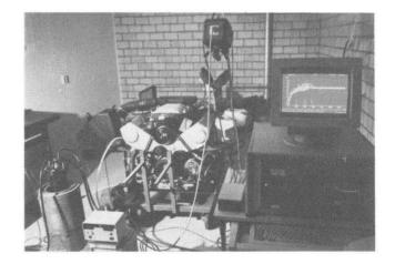
Fig. 3: The wear behavior of Be-7 labelled parts, a gear of Polyamid and a crankshaft seal of Viton (Elastomer), have been measured under real operation conditions in a high-powered engine of Audi on a test bench at the Fa. He $\beta$ , as illustrated by the picture. Demonstration measurements and material testing have been performed in cooperation with the Company Audi and Fa. He $\beta$ , Ingolstadt.
