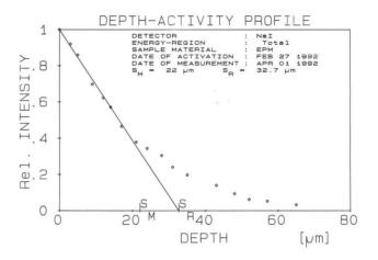
Fig. 2: The activity over depth distribution of implanted Be-7 in EPM-Polyamid is demonstrating the quality of the radioactive labelling by the linear region of 20 µm near the surface suitable for wear measurements.
