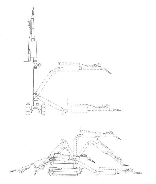
Fig. 1. The basic MRV model demonstrating its dexterity and reach capabilities.
