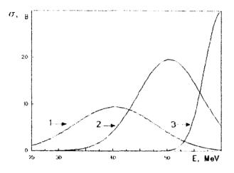
Fig. 2. Calculated excitation functions of the reactions thallium-203 (helium-3,p xn) with radionuclide formation.
