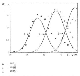
Fig. 1. The excitation functions of the reactions thallium-203 (helium-3,xn) with radionuclide formation. Continuous curves – the results of calculation, the points – experiment: 1 - bismuth-202, 2 - bismuth-201, 3 - bismuth-200.
