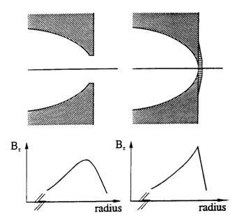
Figure 2 Behaviour of the magnetic field with gap opening and with a magnetic shunt
