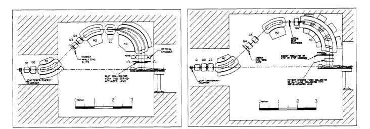
Figure 3 The scanning gantry
