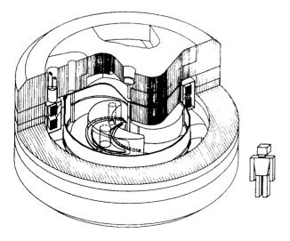
Fig 5 : Cut away view of the superconducting cyclotron and general layout of the SFM synchrotron proposed for EULIMA.
