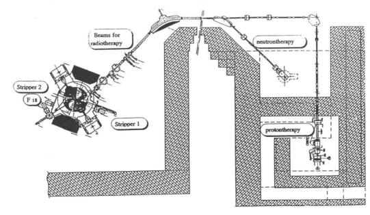
Fig 1 : MEDICYC 65 MEV H<sup>-</sup> cyclotron for neutrontherapy, low energy proton herapy and  $F^{18}$  production.
