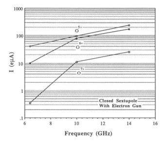
Fig. 3. High charge state oxygen ions produced by the AECR with the closed sextupole magnet and cold electron injection at 6.4, 10, and 14 GHz.
