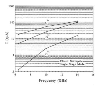
Fig. 4. High charge state oxygen ions produced by the AECR with the closed sextupole magnet operated at a single stage mode at 6.4, 10, and 14 GHz.
