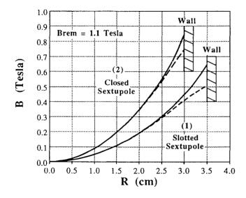
Fig. 2. Two radial field profiles are shown for the AECR. The solid lines show the pole field strength and the dashed lines show the gap field intensity between two adjacent sextupole bars. (1) indicates the case of the plasma chamber with an ID = 7.0 cm (slotted sextupole) and a maximum field of 0.64 Tesla at the chamber wall. (2) illustrates the case of the smaller chamber of ID = 6.0 cm (closed sextupole) and the maximum field strength is increased to 0.84 Tesla.
