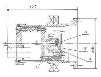
Figure 1: Ion source section
