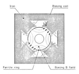
Fig. 2. Principle of ferrite biasing with a quadrupole magnet.
