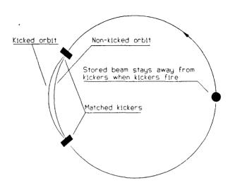
Fig. 6. The low frequency cavity bunches the beam at an azimuthal angle away from the kickers when kickers fire. Lower beam loss can also be achieved by letting beam go through the kickers at the flattop of the kicker pulse.
