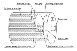
Fig. 3. Cutaway picture of the MPI cavity showing its internal structure.
