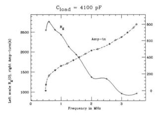
Fig. 4. Bias Ampere-turn and gap resistance versus frequency plot of MPI cavity.
