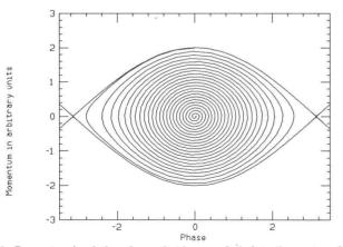
Fig. 1. Computer simulation shows that beam spirals into the center of the rf bucket with combined forces of cooling and rf.
