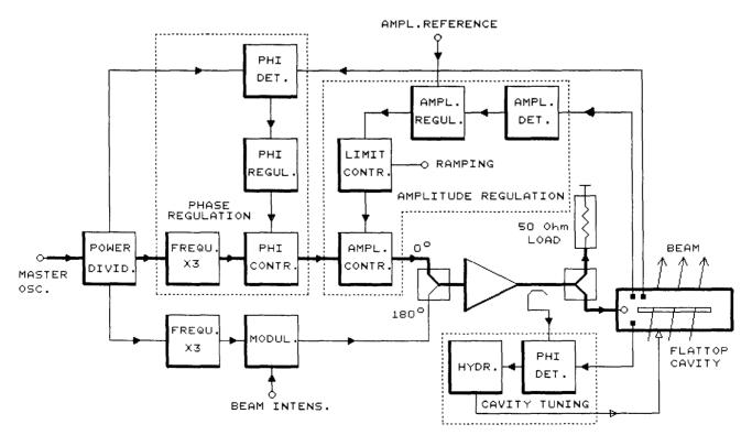
Fig. 2. Simplified block digram of the 150 MHz flattopping cavity control system
