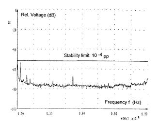
Fig. 1. Cavity voltage rest modulation spectrum, measured on cavity #1, @ I  $_{beam} = 500 \mu A$
