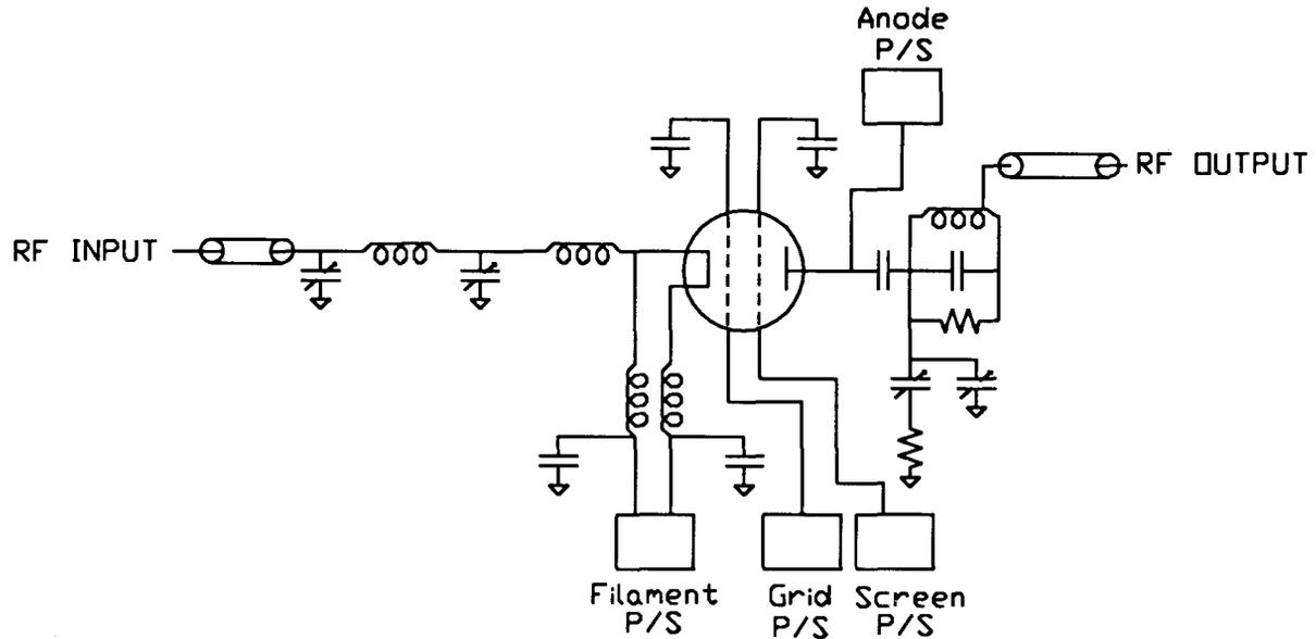
Figure 1. Power Amplifier Simplified Schematic
