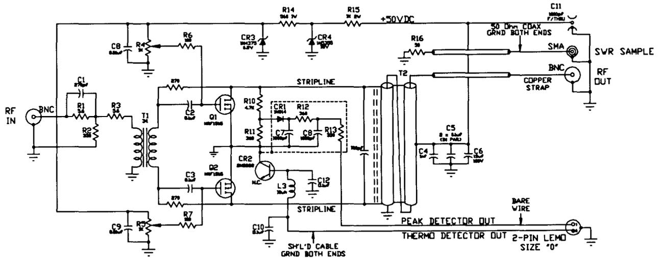
Figure 2. Driver Amplifier Module
