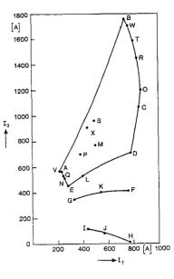
Figure 2. Operating diagram of the AGOR coil system.
