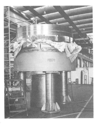
Figure 1. The AGOR cryostat during assembly.
