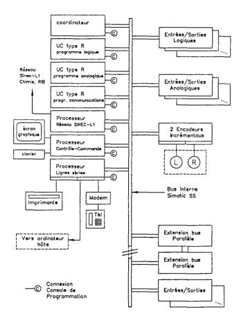
Fig.7: SIMATIC-S5 system as implemented for CY-CLONE 30. The system also provides 2 shaft encoders to fine-tune parameter settings.
