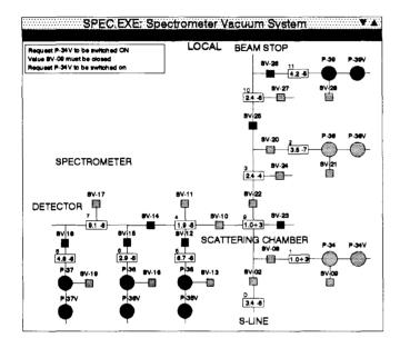
Fig. 3. A copy of the colour monitor video display of the spectrometer vacuum system.
