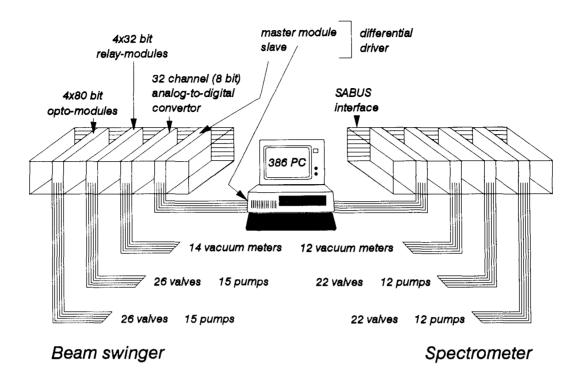
Fig. 1. A scematic view of the instrumental node for the two vacuum systems.
