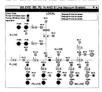
Fig. 2. A screen copy of the colour monitor video display of the 'beam swinger' vacuum system.
