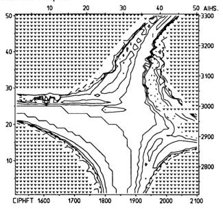
Fig. 6. A twodimensional scan of flattop phase and main magnet excitation recording extraction losses. The strange shape of the domain where scanning is possible reveals the advantage of a program that finds this domain automatically.
