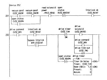
Figure 2. Section of ladder logic code. A processor bit is represented as a relay with an arbitrary number of contacts.
