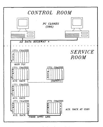
Figure 1. Overview of the Control System Hardware Configuration
